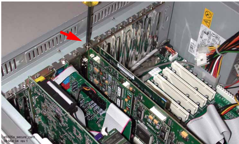
Figure 320 Secure card with screw
