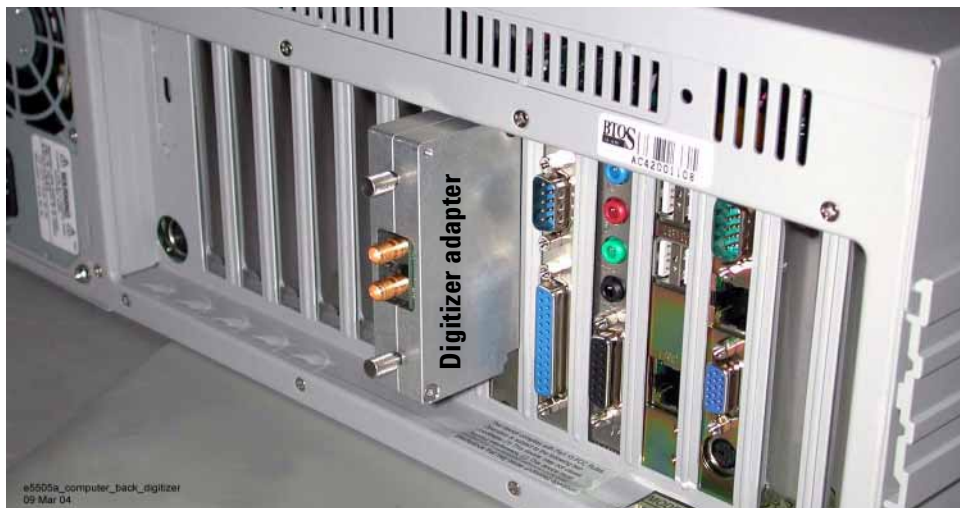
Figure 304 Connect adapter to PC digitizer card
