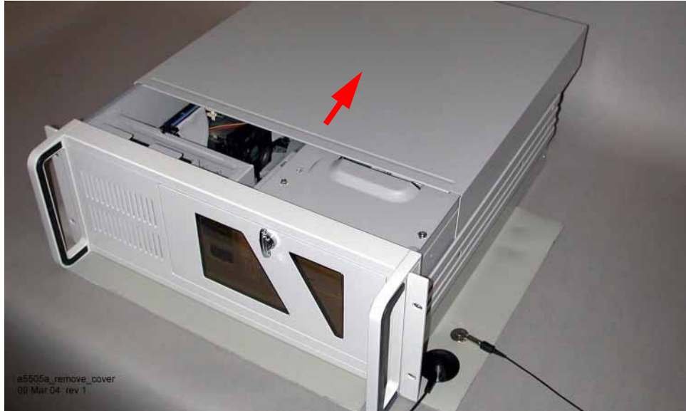
Figure 311 Slide cover off
