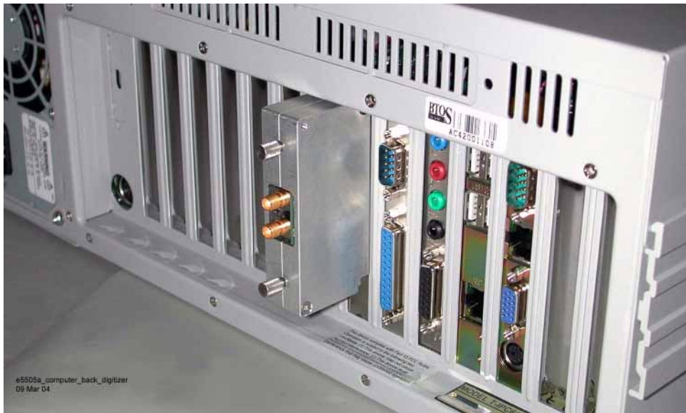
Figure 317 Connect adapter to PC digitizer card
